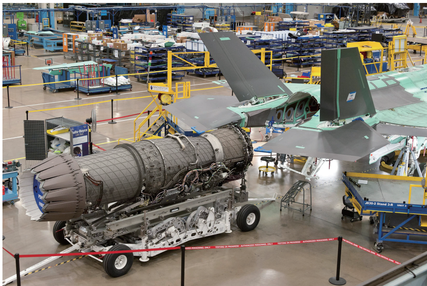
图1 F-35战斗机发动机整机安装 Fig.1 Aeroengine installation of F-35 fighter
